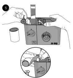
Open the lid and, while being careful not to pull out the film, remove the spool, the backing paper excess and the adhesive from the film.
