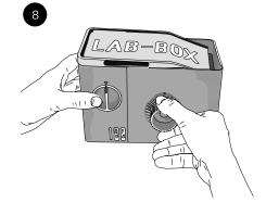
Turn the tank knob in order to wind the film onto the reel. Now you can start processing your film.
