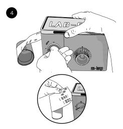
Turn the 120 knob counter-clockwise into closed position (square symbol). Now you can tear away the paper.
