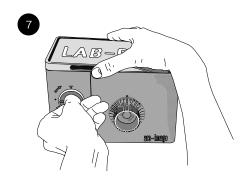
Close the lid and turn again the 120 knob (triangle position) to open the lightproof chamber and relase the film.
