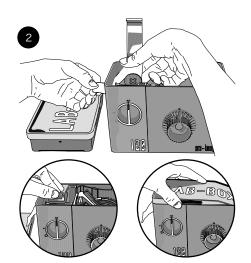
Insert the black backing paper in the rear split and place the roll in the film slot. Then close the grey block and close the lid.
