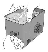
Now, push up the grey lever on the back to cut the film from the cartridge.
