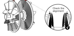
Check again that all the elements are properly aligned and that the bla de is not visible.
