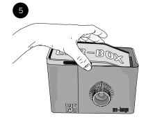
Close the lid and turn the tank knob in order to wind the film onto the reel.
