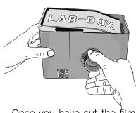
Once you have cut the film, tùrn the knob in order to wind the last part of the film onto the reel. Now you can start processing your film.
