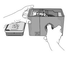
Turn the tank knob until the hooked film starts to slide correctly though the film guide.
