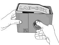
Once you have cut the film, turn the knob in order to wind the last part of the film onto the reel. Now you can start processing your film.
