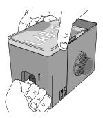
Now, push up the grey lever on the back to cut the film from the cartridge.
