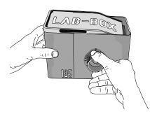
When the tank knob stops turning, it means you have reached the end of the roll.
